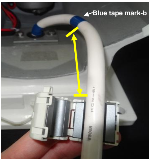
11) Attach the ferrite core from blue tape-b to 10cm end.
