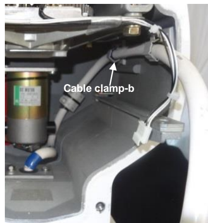
14) Clamp the cable by the cable clamp-b.
